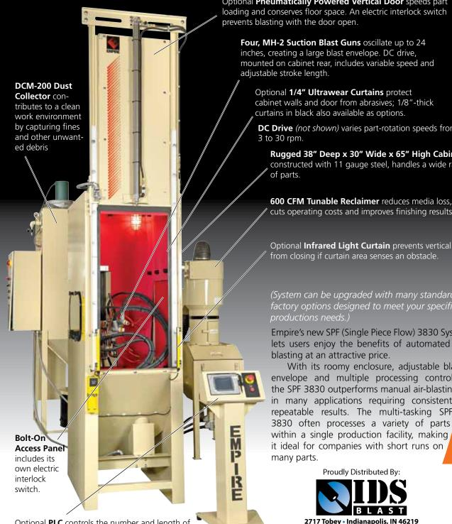
Optional PLC controls the number and length of guns oscillations. (Standard control panel mounts on the left side of the cabinet in place of the viewing window.)
